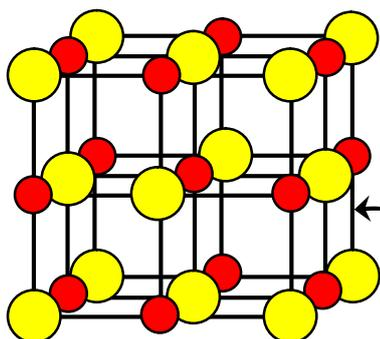
Above: the giant ionic lattice of NaCl – which spheres represent the sodium ions (large or small)?
